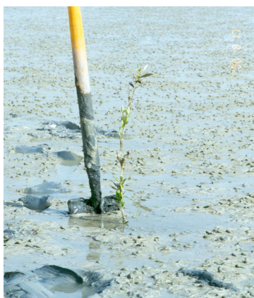
Plate 71. Shovel penetration showing the depth of the muddy layer near a live plant at the Shuwaikh (KISR) Site, Subsite C.
