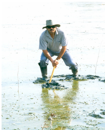
Plate 65. Penetration of a shovel without any restriction showing the absence of gravels in the lower muddy Zone in the Shuwaikh (KISR) Site, Subsite A.
