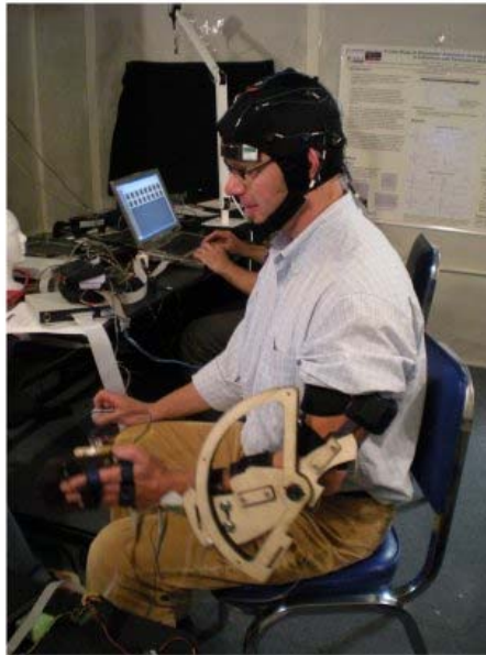
Brain Cap, a non-invasive, sensor-lined cap
