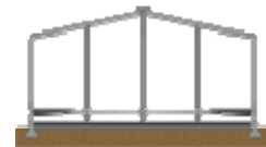
Internal Floating Roof
