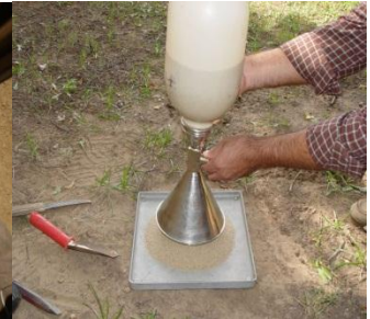
Sand cone test
