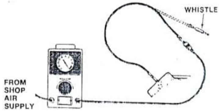
**Fig. 8.6 Cylinder – leakage tester. The whistle is used to locate TDC in cylinder No. 1
