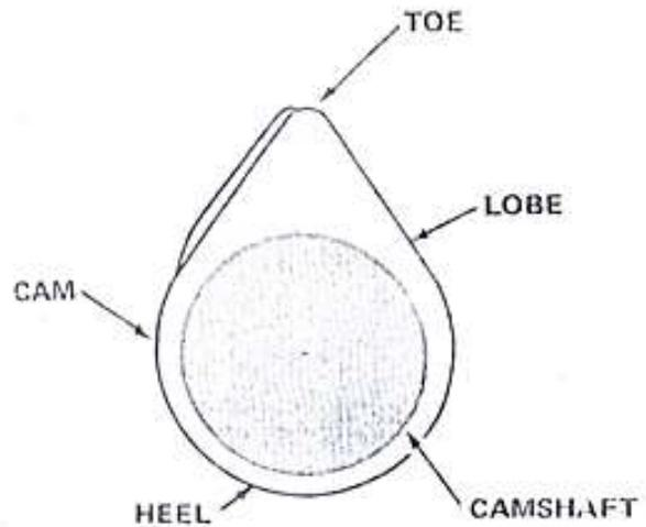
Fig. 8.1 Cam on a camshaft. Note positions of the toe and heel.
