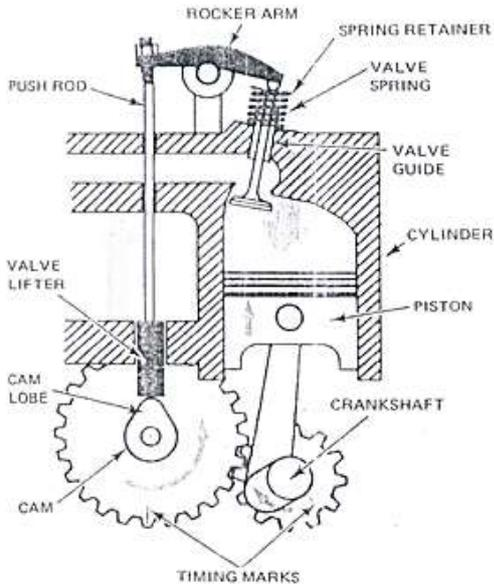
Fig. 8.2 Valve train on an engine using a pair of gears to drive the camshaft. The cam lobe has pushed the push rod up so the valve is opened.
