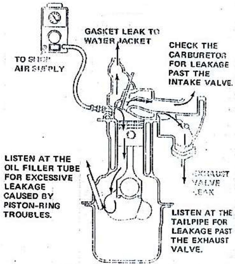
**Fig. 8.7 How the Cylinder – leakage tester works. It applies air pressure to the cylinder through the spark – plug hole with the piston at TDC and both valves closed. Points where air is leaking can be pinpointed. (Sun Electric Corporation)**
