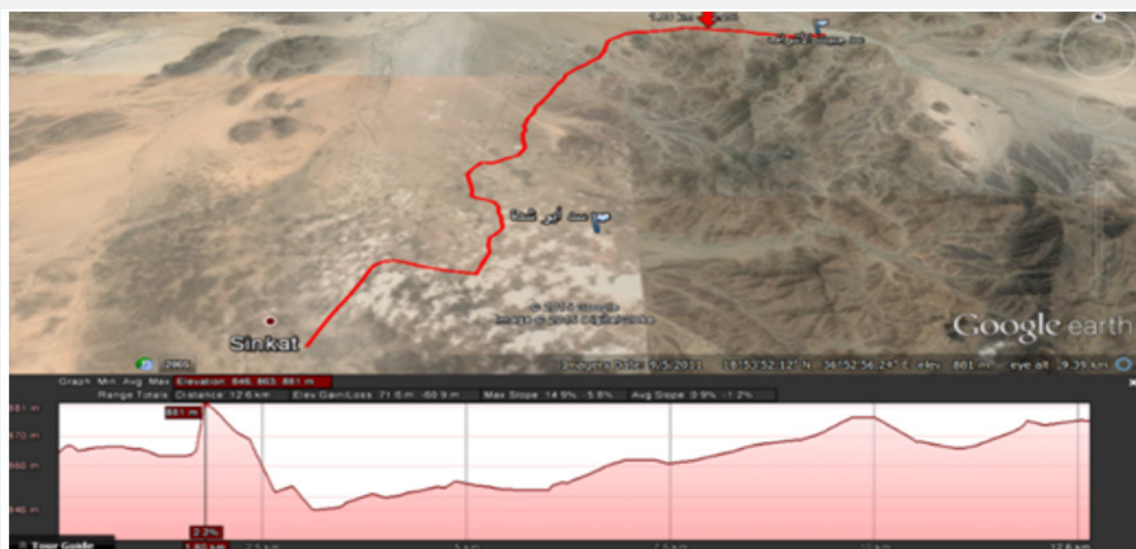
Figure 2: Water pipeline from Gebeit Dam to Sinkat town.
