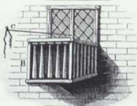
Trap of Pigeon-lift. Interior showing the loose bars called "the bolt." B, the little swinging doors on the inner end. C, the string which pulls up the outer door.
