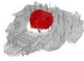
main auditorium spatial steel structure
