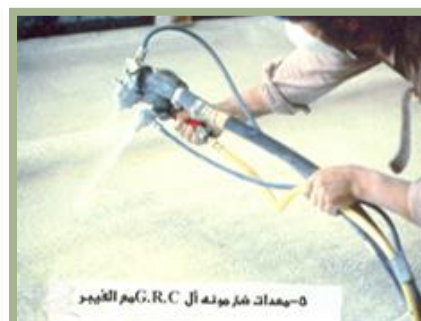
7-spray-gun-for-premixing pumping
