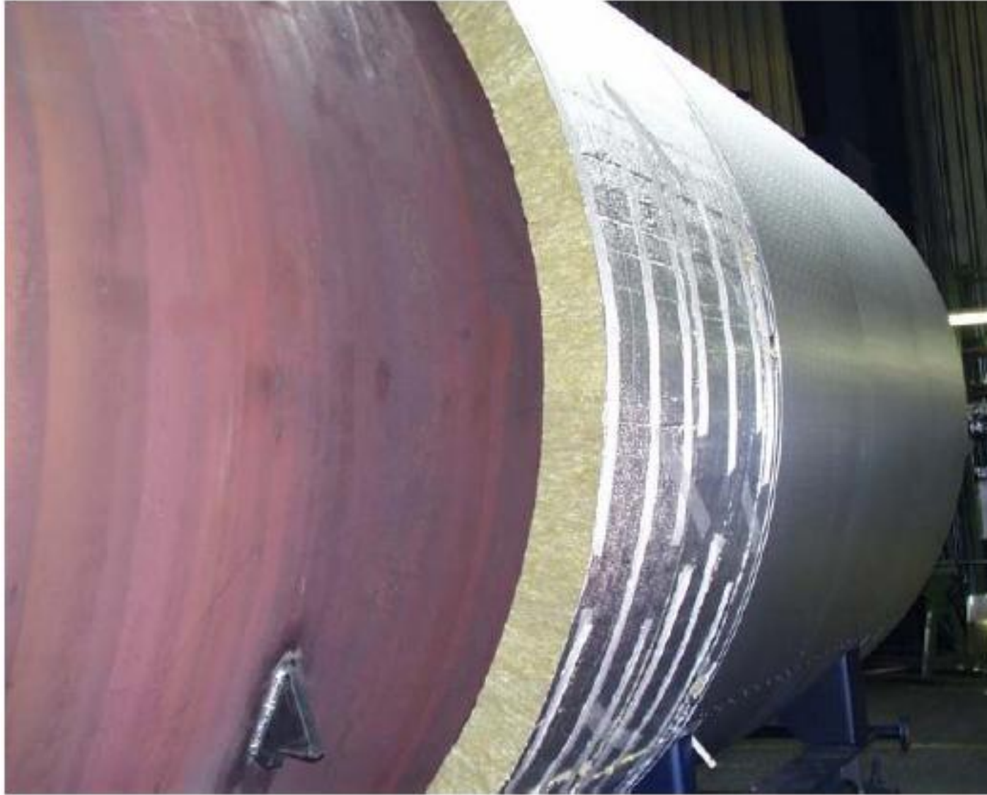
Factory photograph of a boiler during insulating without spacers in the cylinder area
