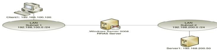
Figure 9-1 Routing two subnets
