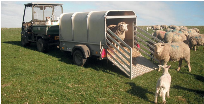
Fig 31 A stock trailer can be made by adding a top to a low-sided trailer. A one-piece demountable top leaves the trailer available for general use. The back hinges down to provide a ramp. Sides should be solid, with ventilation gaps at the back and front just below the roof. If the ramp is shiny and spooks the sheep, cover it with a piece of carpet. A low, removable partition can be sited at the front of the trailer to keep small lambs separate from ewes.
